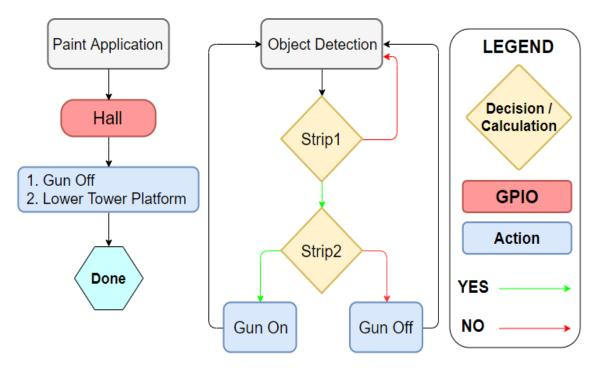
Figure 7.3: Paint Application & Object Detection
