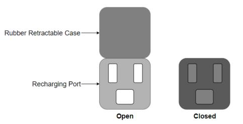
Figure B.6: Recharging Port - Rubber Retractable Case
