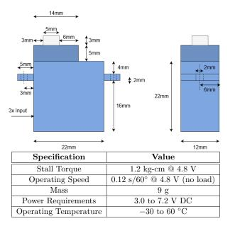
Figure 2.2: Wheel Pivot Motor [3]
