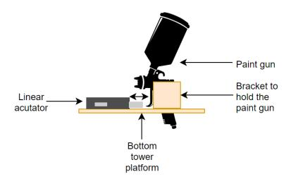
Figure 4.9: Trigger Mechanism Design [25]
