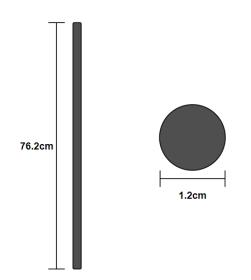
Figure 4.3: Tower Support Beam [22]
