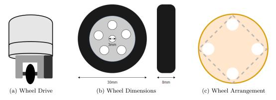
Figure 2.1: Wheel Drive & Arrangement
