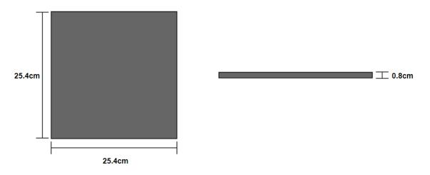
Figure 4.4: Tower Platforms Dimensions
