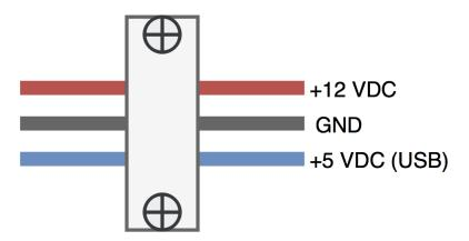
Figure 6.2: Wiring Appearance
