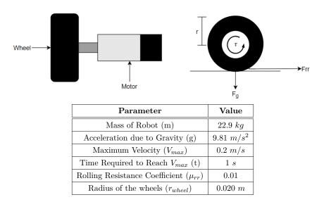
Figure 2.3: Drive Motor & Wheel [4]
