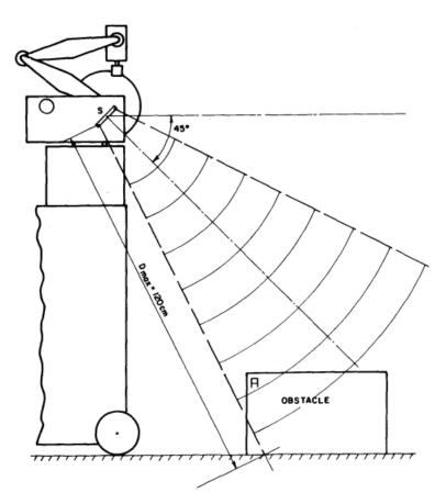
Figure 3.3: Ultrasonic Rangefinders for Obstacle Detection [18]
