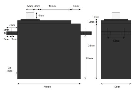
Figure 4.8: Tower Pulley Motor [6]
