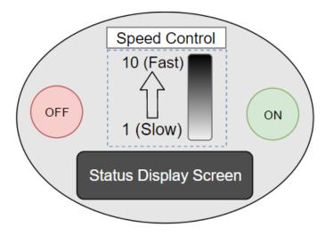
Figure B.2: User Interface Buttons & Switch
