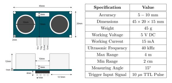
Figure 3.4: Ultrasonic Rangefinder [19]
