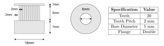
Figure 4.5: Tower Pulley System Gear [24]
